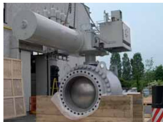
48" Class 600 valve with Electrohydraulic actuator
