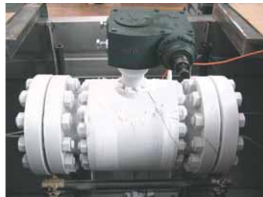
Cryogenic testing on an 8" (20 mm) class 300 valve.
